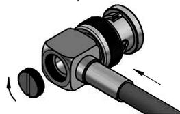
**Step 5.** Crimp ferrule with tool hex size : .213" (check point 4)
